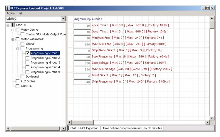
The project displayed here is interesting because it displays the applicationming parameters of a motor drive 160 SSC. It also displays topics from a PLC.
