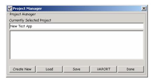
The "iMPORT" button has a special function. Project files have a specific file format. If you decide to edit the project in Excel you will need to use the import function to put the file back in the correct format. See "File format" for specifications of the project file format.
